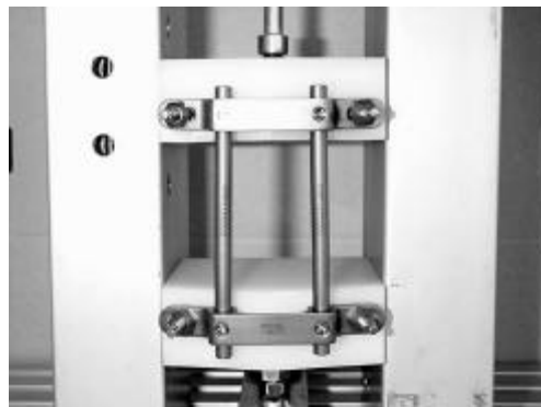
Fig.2: Test setup for the determination of the mechanical strength of an internal fixator.
